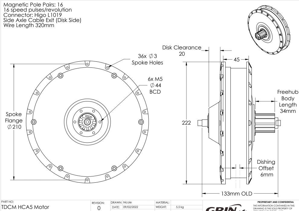
Rear Hub Motor with Torque Sensor
